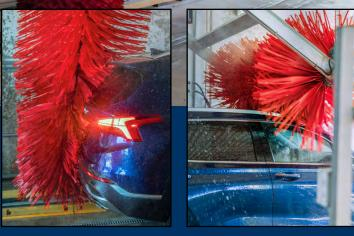
Intelligent programming senses vehicle speed and profiles accordingly
